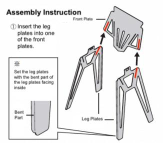
② Insert the second front plate into the leg plates simultaneously on both sides. Please note that both side must be inserted at the same time or they will not fit.
