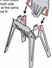
(3) Insert side plates into the slit parts in front plates.
